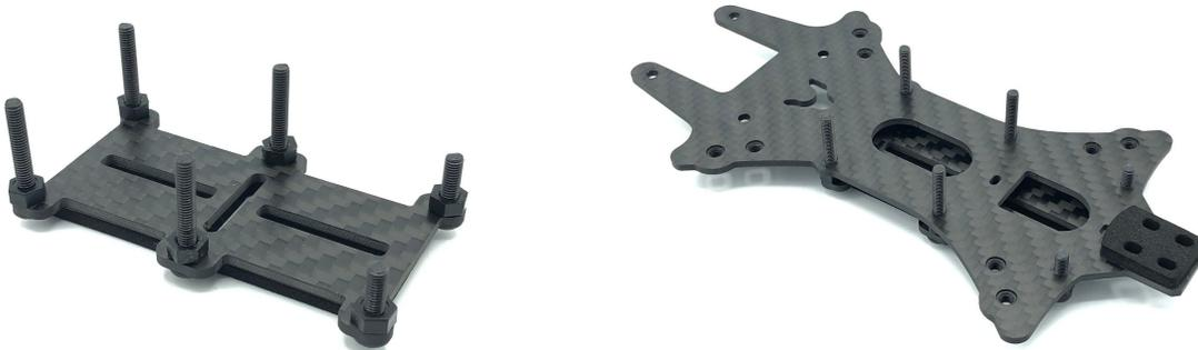
**Using 4 x 8mm bolts, install 2 x 10mm standoffs up front along with TPU cam mounts, and 4 x 15mm standoffs as shown. The slide TPU shelves over standoffs and mounting bolts**
