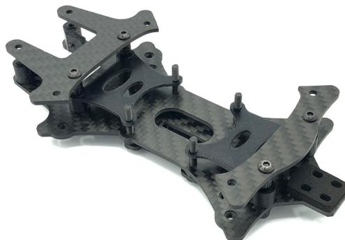
Pay attention to arm orientation and slide them along with the 5mm carbon spacers into their mounting areas. The carbon spacer **MUST** be underneath the front arms if installing the front braces. Using 4 x 22mm bolts attach the arms and carbon locks to the body.
