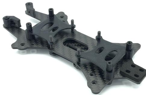
**Add 4 x 8mm to secure the front and rear bottom plate sections to the rear four standoffs. Don't tighten all the way yet.**
